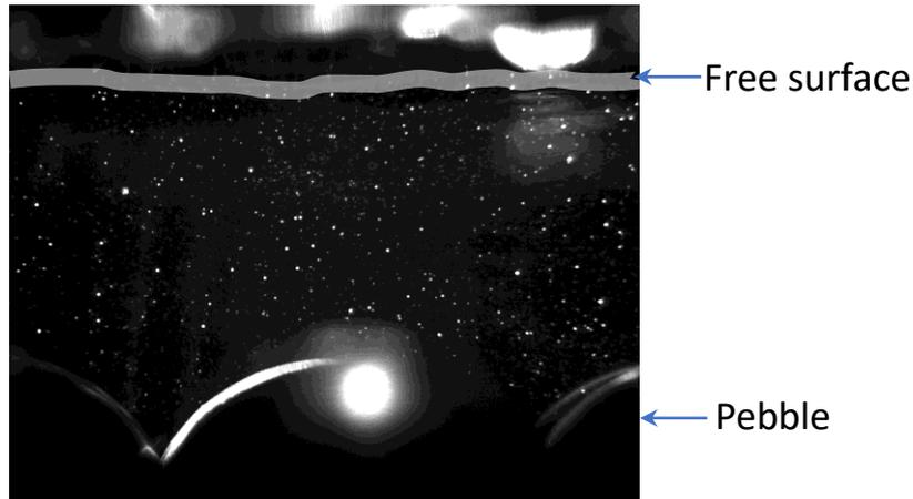
Fig. Particle image of PIV
