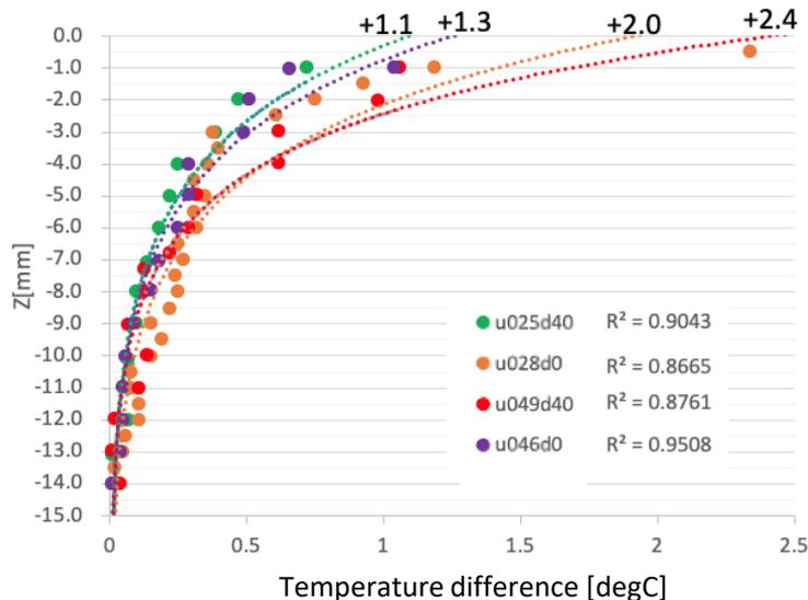
Fig. Surface temperature increase (X=0)
