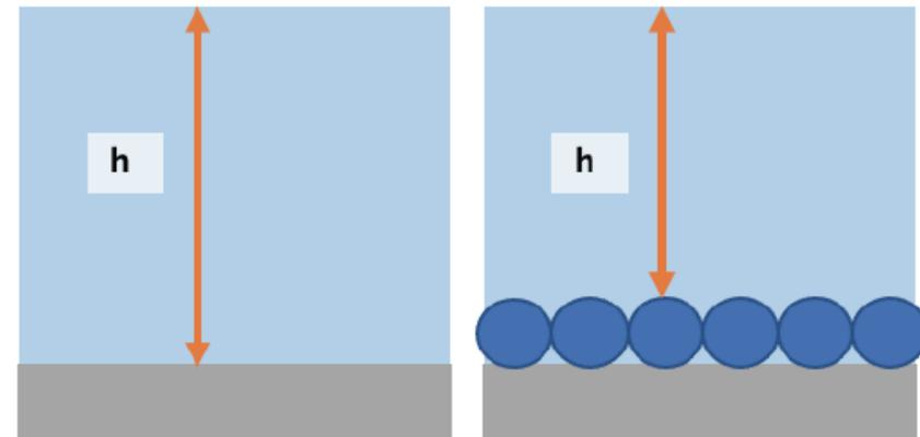
Fig. Definition of the h(flow film definition)
