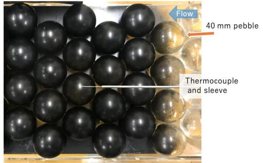
Fig. Location of the thermocouple ( $x, y=0$ )
