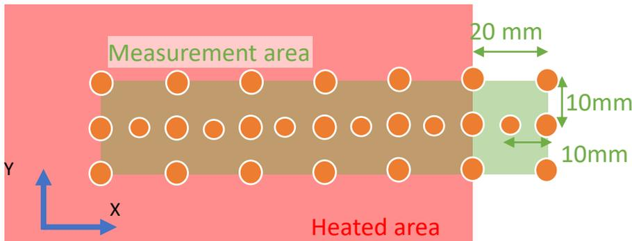
Fig. Location of the measurement points
