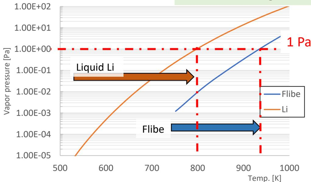
Fig. Vapor pressure of Flibe and Li [2] [3]
