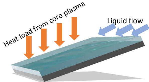
Fig. Image view of liquid divertor
