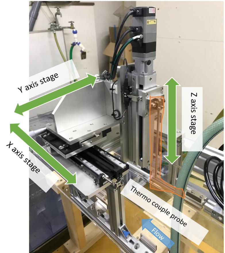
Fig. Picture of the XYZ stage temperature measurement unit
