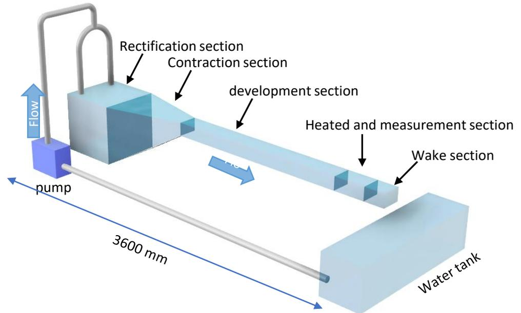
Fig. Image view of the experimental water loop
